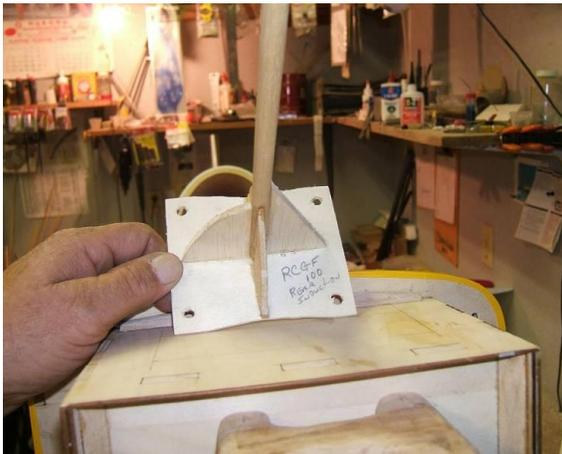
No matter what engine you elect to use on any plane, a basic mounting template can be home made out of a length of 3/8" or whatever wood dowel long enough to reach from the firewall through the cowl ring, a piece of 1/8" plywood, and some 1/8" balsa sheet triangle gussets. That's it, that's all, and you have an engine template that can be used on any plane you choose to use that engine on. You only need to determine the engine mounting
