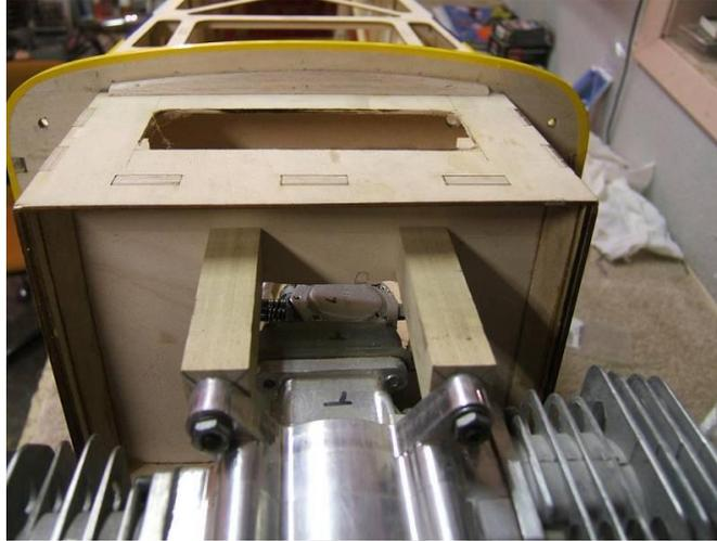
No need to glue them to the aircraft firewall unless you want to but that makes it a bit tough to change to another engine type at some later date. I prefer the structural rigidity that a "boxed" engine mount provides. No engine twist as you would have with individual standoffs. Nada, nyet, none! You can box the entire mount or simply add a sheet of ply to any pair of legs. No movement at all and much more secure than individual aluminum standoff legs.
