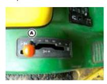
Move the throttle lever (E) all the way up (Choke position)
